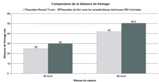
In addition, the EBS system has been calibrated with Renault Trucks brake pads. Using any other brake pad can result **in even longer braking distances**.
