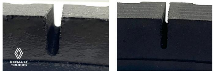
It was also noted that the ears of some adaptable parts are less strong and therefore would break more easily. This would lead to more noise / vibration, increased risk of parts breaking and reduced service life.
